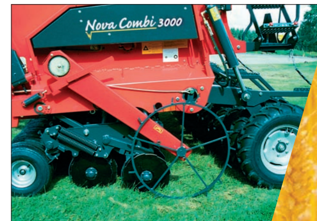
The feeder in Nova Combi is used with a ground wheel
